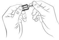
Insert blade into the mini hand driver hole
